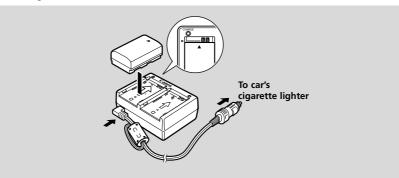
• Fast charging for the high-capacity BP-522 and BP-535 (both optional). 15 minutes of charging gives 60 minutes of recording (using the viewfinder).
